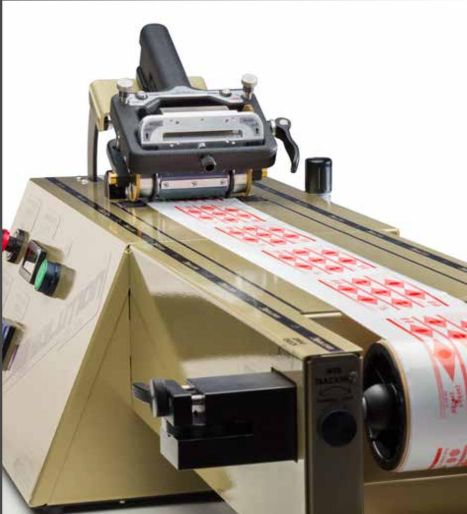
Since first introduced in 2002, the Perfect Proofer® automated ink proofing system has evolved several times – with each model incorporating successive generations of new technology. Today, the system lets process control specialists use Dot Gain Technology™<sup>1</sup> to preview exactly how any ink formulation will reproduce on the press for which it's intended. Any substrate; UV, water- or solvent-based inks; all can be previewed equally well.
